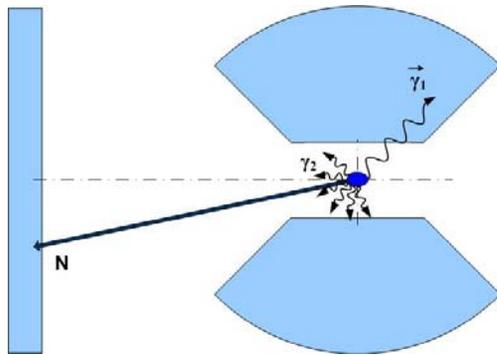
Asymmetric decays: If the first photon is emitted at **the backward angles**, the low-energy second photon can be detected in the Russian Wall or the BGO Ball.
