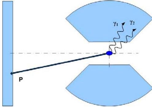
Symmetric decays are rejected by the analysis of cluster shapes in the BGO Ball. Efficiency of this rejection is  $\sim 99\%$ . If the pion is emitted at backward angles, its energy is low. Such events are suppressed.
