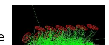
12 Nordball liquid scintillators were placed around the Active Target to detect neutrons coincident with charged recoils in the target. They were placed a flight path of  $\sim 1.5$  m.
