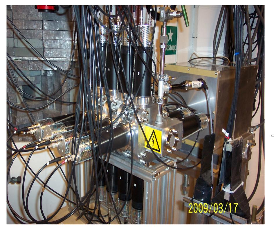
The Active Target is a helium gas scintillator where the target "Helium" also act as a detector of particles generated Pressure gage Red Balzers 50bar ressure gage
