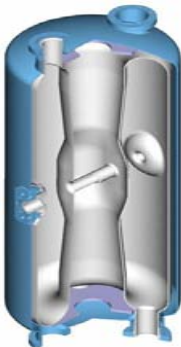
Half-Wave Resonator (HWR)
