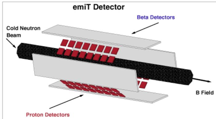
(Top) Schematic of the emiT apparatus. The beta detectors are plastic scintillator, the proton detectors consist of arrays of surface barrier diode detectors. (Right) Histogram of coincidence events. The peak is due to neutron decay.
